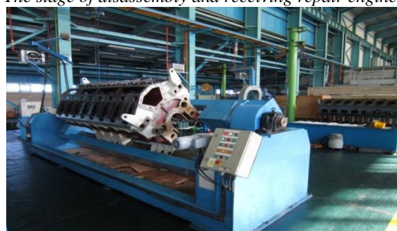
Turnover station to enhance assembly and disassembly activities
