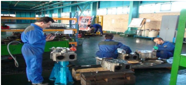
Disassembly, washing, component inspection, NDT on firing surfaces, leakage test, seating valves, etc.
