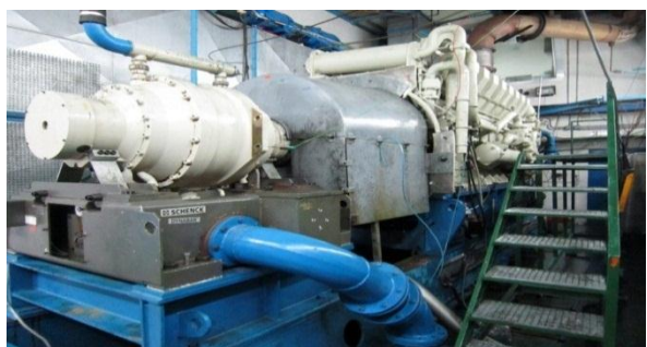
Sending the engine to test cell, installing electrical and mechanical joints, engine loading based on test procedures
