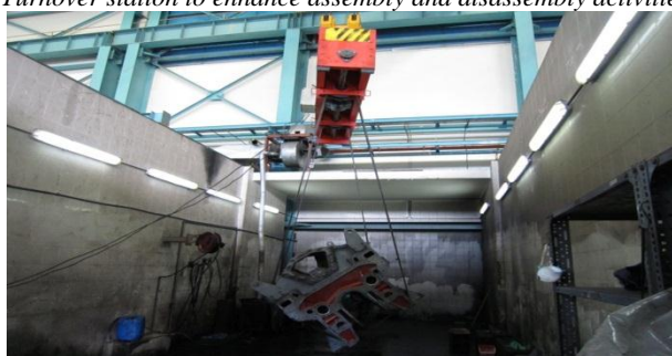
Engine block turnover tool to wash and inspect different sections
