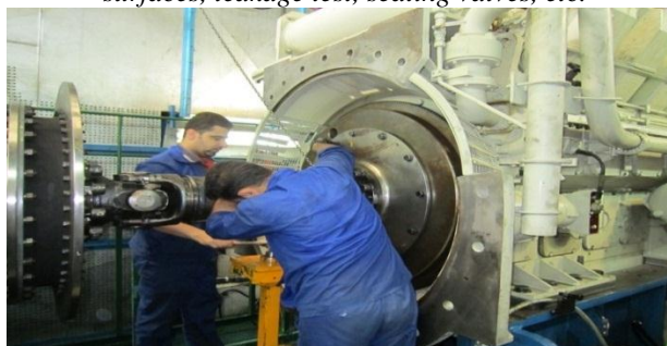
Sending the engine to test cell, installing electrical and mechanical joints, engine loading based on test procedures
