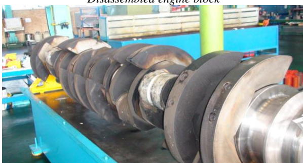
The stage of cleaning all bearing seating surfaces and crankshaft oil drillings
