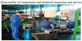
Disassembly, washing, component inspection, NDT on firing surfaces, leakage test, seating valves, etc.
