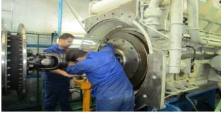
Sending the engine to test cell, installing electrical and mechanical joints, engine loadind based on test procedures
